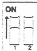
Figure 6-3. Floppy Diskette Drive Address Switches
